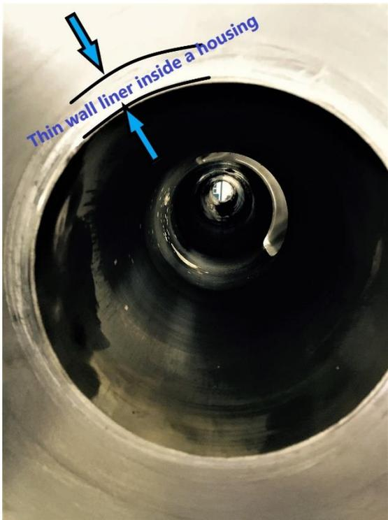
There are many well documented problems with this method. The strength of the barrel is now compromised as compared to a single piece construction method. The thermal heat transfer from the outside heater bands to the melt stream inside the barrel has now been reduced since there are gaps between the liner and housing.
