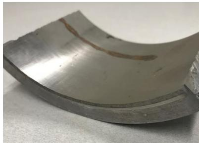
*Specimen from Imported Barrel which was a thin walled liner pressed into a housing*
