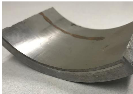
Exhibit C: Specimen from 135mm Imported Barrel which was a thin walled liner pressed into a housing
